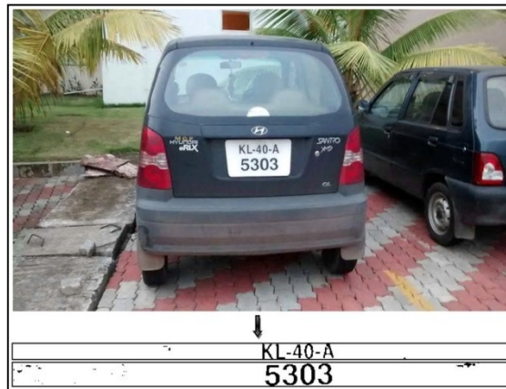
Figure 17. Successful Extraction of Double Lined Number Plate
