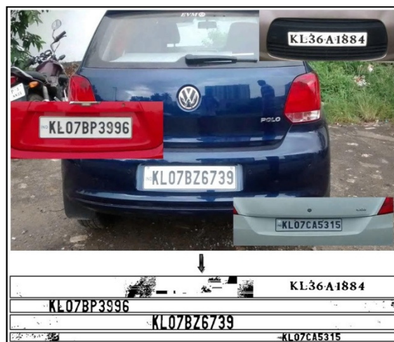
Figure 18. Detection of Multiple Number Plates from Single Input Image
